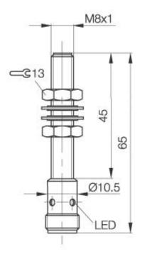
Inductive Sensors BES M08MH1-NSC15B-S04G M 8 x 65 normally-open Sn=1,5mm shielded
